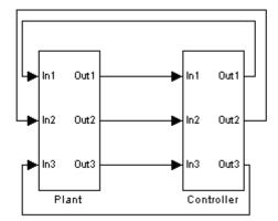
Your starting point in developing a plant/controller system is to model the system as two subsystems in closed-loop simulation. As your design progresses, you can use Simulink external mode with standard Real-Time Workshop targets (such as GRT or ERT) to help you model the control system separately from the plant.
